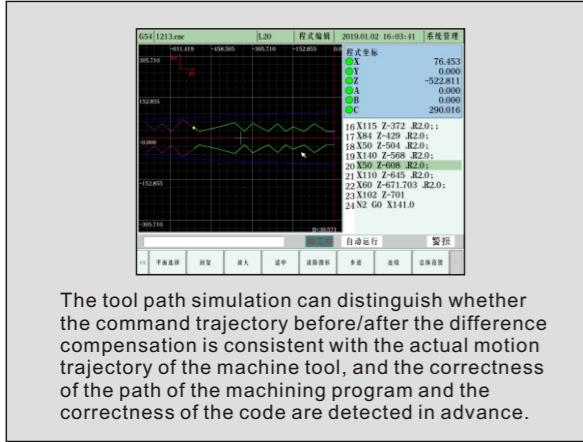
The tool path simulation can distinguish whether the command trajectory before/after the difference compensation is consistent with the actual motion trajectory of the machine tool, and the correctness of the path of the machining program and the correctness of the code are detected in advance.
