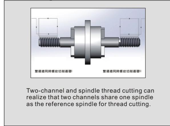
Two-channel and spindle thread cutting can realize that two channels share one spindle as the reference spindle for thread cutting.
