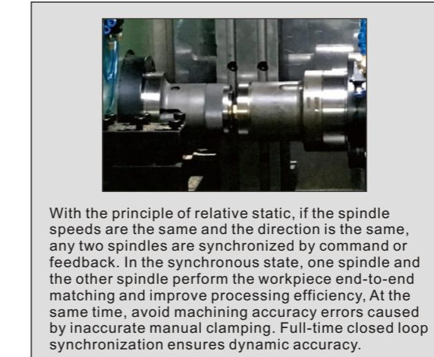
With the principle of relative static, if the spindle speeds are the same and the direction is the same, any two spindles are synchronized by command or feedback. In the synchronous state, one spindle and the other spindle perform the workpiece end-to-end matching and improve processing efficiency. At the same time, avoid machining accuracy errors caused by inaccurate manual clamping. Full-time closed loop synchronization ensures dynamic accuracy.
