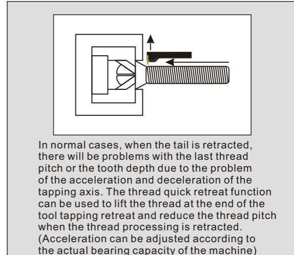
In normal cases, when the tail is retracted, there will be problems with the last thread pitch or the tooth depth due to the problem of the acceleration and deceleration of the tapping axis. The thread quick retreat function can be used to lift the thread at the end of the tool tapping retreat and reduce the thread pitch when the thread processing is retracted. (Acceleration can be adjusted according to the actual bearing capacity of the machine)
