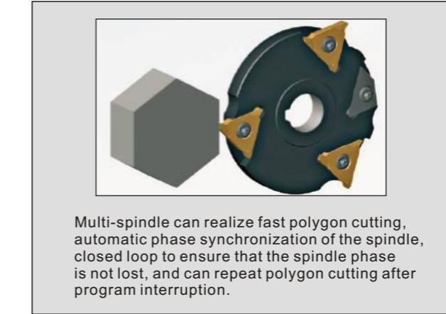
Multi-spindle can realize fast polygon cutting, automatic phase synchronization of the spindle, closed loop to ensure that the spindle phase is not lost, and can repeat polygon cutting after program interruption.
