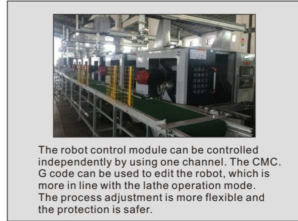
The robot control module can be controlled independently by using one channel. The CMC. G code can be used to edit the robot, which is more in line with the lathe operation mode. The process adjustment is more flexible and the protection is safer.
