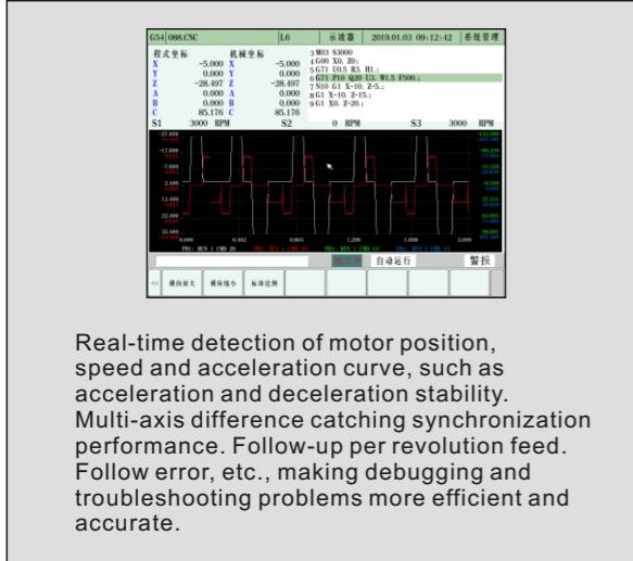
Real-time detection of motor position, speed and acceleration curve, such as acceleration and deceleration stability. Multi-axis difference catching synchronization performance. Follow-up per revolution feed. Follow error, etc., making debugging and troubleshooting problems more efficient and accurate.
