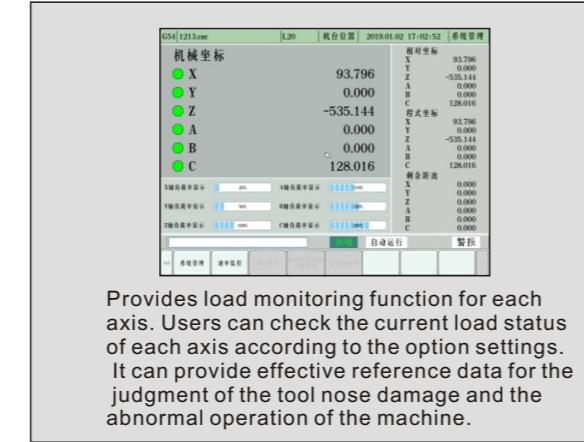
Provides load monitoring function for each axis. Users can check the current load status of each axis according to the option settings. It can provide effective reference data for the judgment of the tool nose damage and the abnormal operation of the machine.
