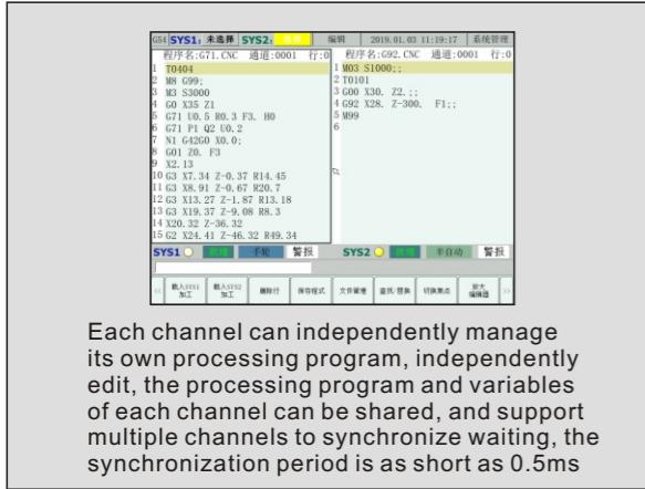
Each channel can independently manage its own processing program, independently edit, the processing program and variables of each channel can be shared, and support multiple channels to synchronize waiting, the synchronization period is as short as 0.5ms
