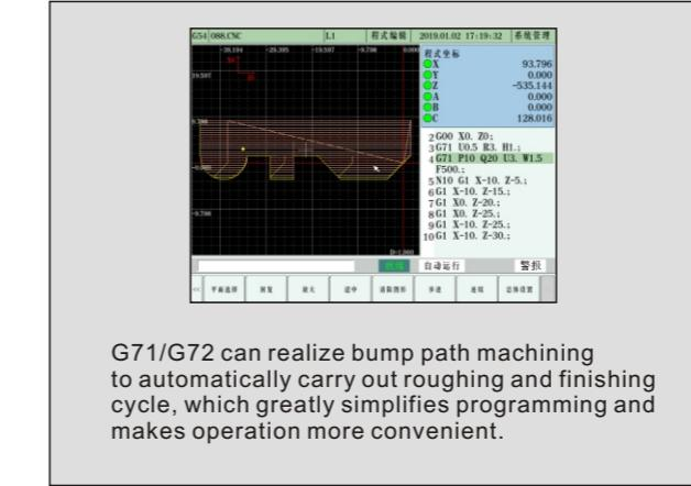
G71/G72 can realize bump path machining to automatically carry out roughing and finishing cycle, which greatly simplifies programming and makes operation more convenient.
