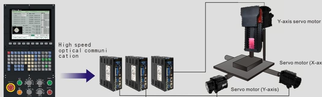
Vertical CNC interface with high-speed spindle motor. Tapping precision and high speed, can also be used with multi-spindle to tap and improve processing efficiency.
