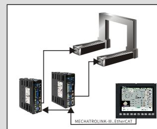
The gantry synchronous axis function can simultaneously perform the displacement of multiple pairs of feed axes without mechanical deviation. The system can quickly process the closed loop control of the synchronous axis and support the absolute value serial bus encoder such as SSI to improve the performance and efficiency of gantry synchronous control.
